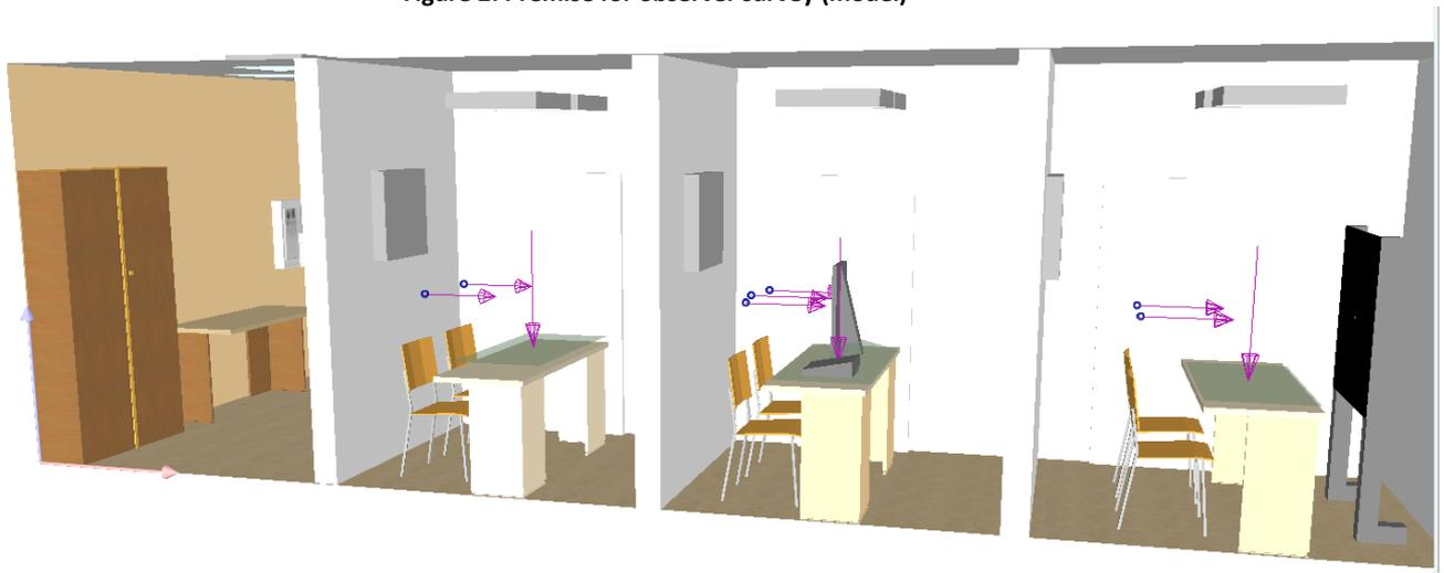
Figure 3: Experimental premises. UGR checkpoint placement for observers and horizontal operation surfaces in experimental areas
