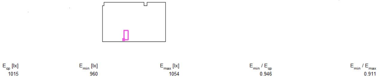
**Figure 6: Distribution of light and its unevenness at the lighting with two CapFlat 66-16 ( $T_{UB} = 3045$  K) lights.**
